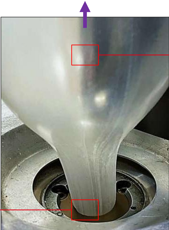
CONSTAB laboratory blown film: C4-Zn-LLDPE 5 kg/h, die 25 mm, gap = 0,2 mm, mono-layer 60 μm
